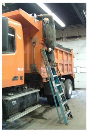
An accident waiting to happen! Stepladders should never be leaned against a truck body and used like a regular ladder.
